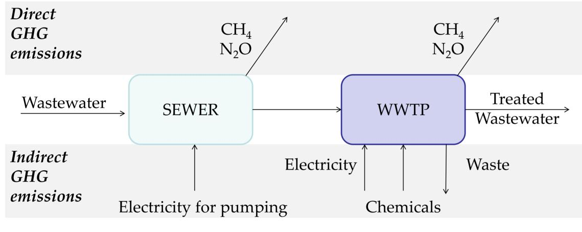
*Figure 1. Diagram of the system boundaries*
